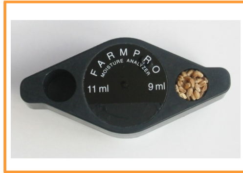
Figure 1a. Fill the measuring cup to the top, ensuring the crop is level with the top of the grinder/compressor cap.
