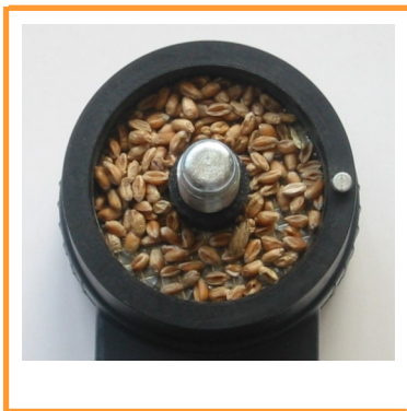
Figure 1 b. Pour measured sample into measuring cell. Note: Stainless steel stop pin on right-hand side of cell
