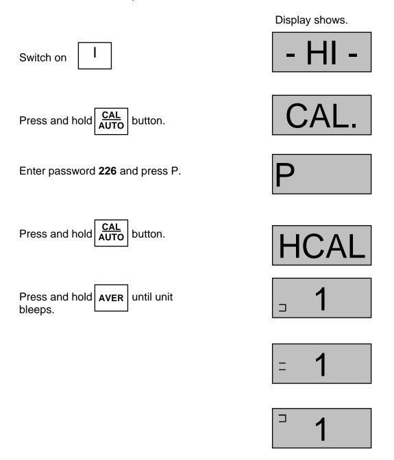
Surround the sensor with a capacitance reference sample (e.g. 28.1). Allow 1 minute for the sensor and sample temperature to equalise. Enter Reference Value (e.g. 28.1).
