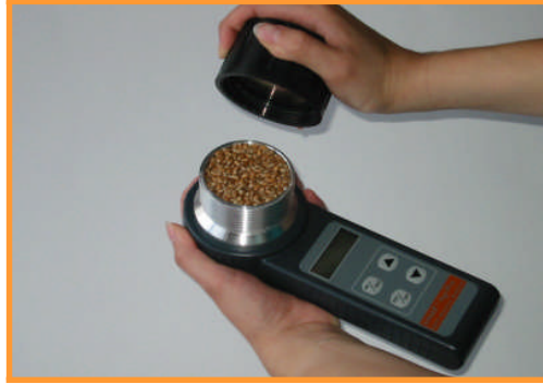
Figure 1a. Fill the measuring cell evenly to the top, ensuring the crop is level with the top of the cell. Screw on the cap and tighten until the stainless steel pressure indicator is flush with the top of the cap.
